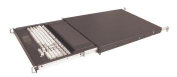
Carefully lift the LCD display into a suitable viewing position. Now gently slide the drawer back to a comfortable position.
